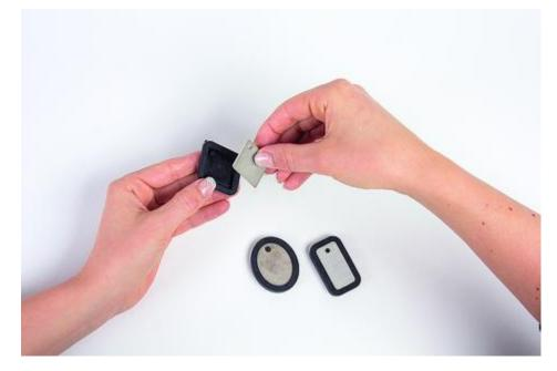
The **temperature** and **humidity** are decisive for the drying time. However, it is advisable to remove the trailer from the mould the **next day**. The upper side, i.e. the later back side, can be dried with a fine **Sandpaper** straightening and smoothing.
