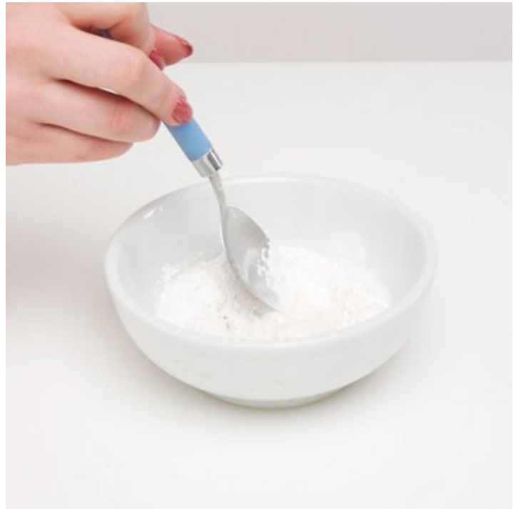
2. Mix casting powder and water to a liquid mass
